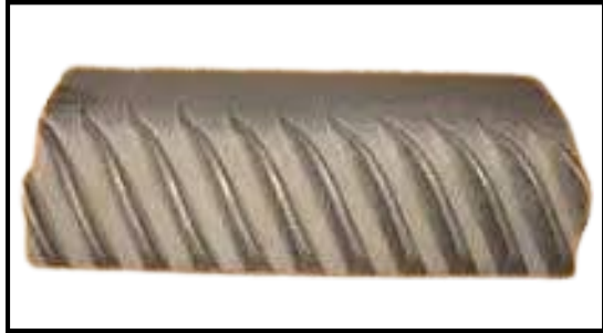
Hard Chromed without polish Teeth hardness (58-61 HRC)
